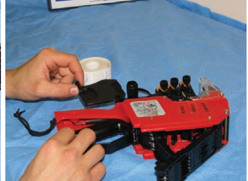
3. Open label roll holder & insert label roll. Feed label strip through applicator.
